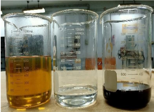
Fig. 1. Appearance of diesel, n-pentanol and waste cooking oil.
