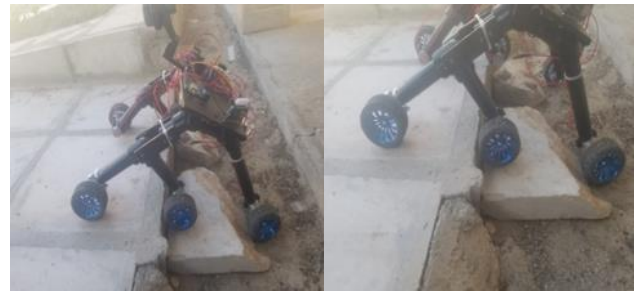
Fig. 10. climbing action of rover
