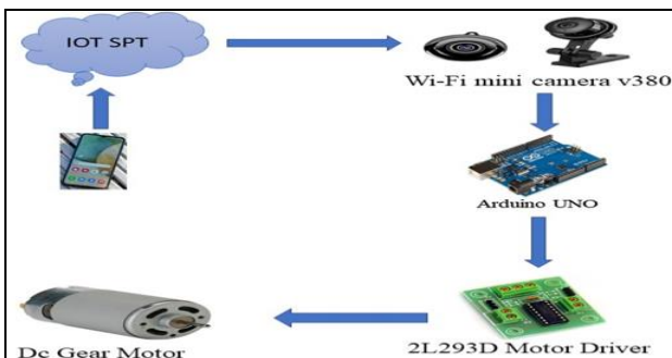
Fig. 3. Block diagram showing working mechanism of rover
