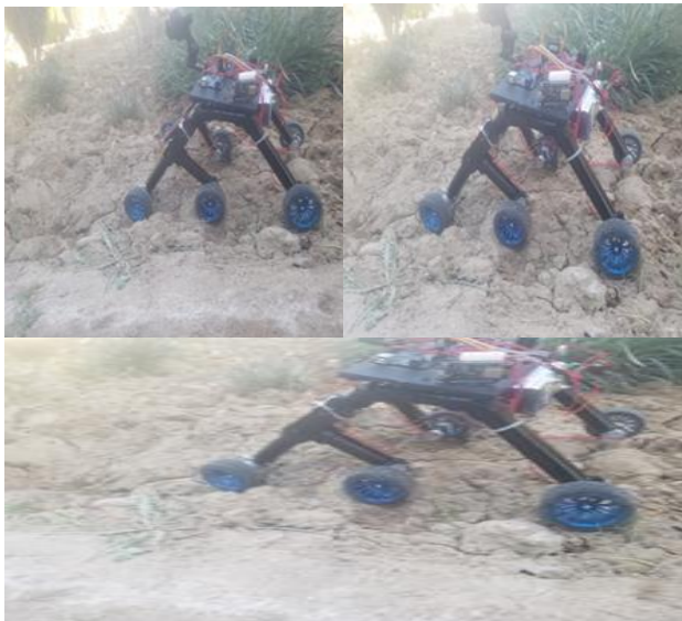
Fig. 8. Rover moving on rough and wet surfaces
